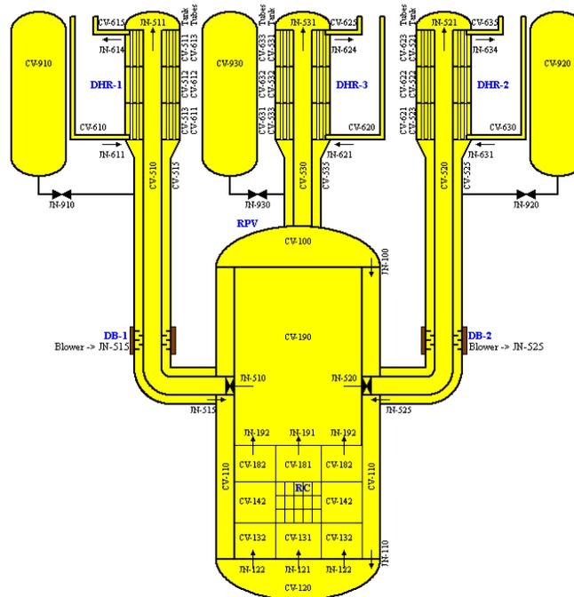
Fig 4 DHR loops with  $\text{CO}_2$  tanks.
