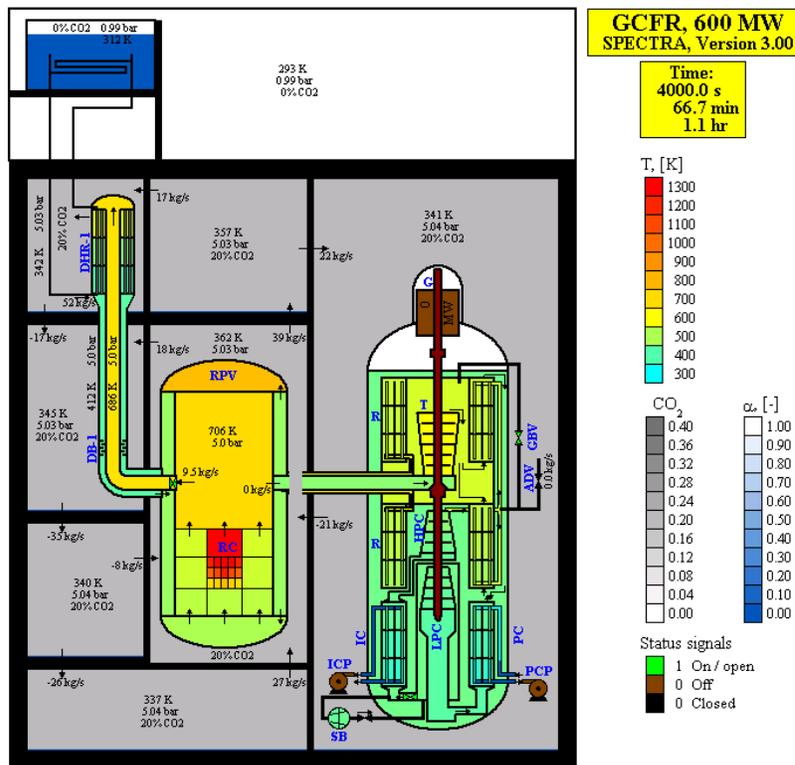
**Fig 9 Containment CO<sub>2</sub> concentrations at t = 4000 s. PCU duct rupture, Case 3.**
