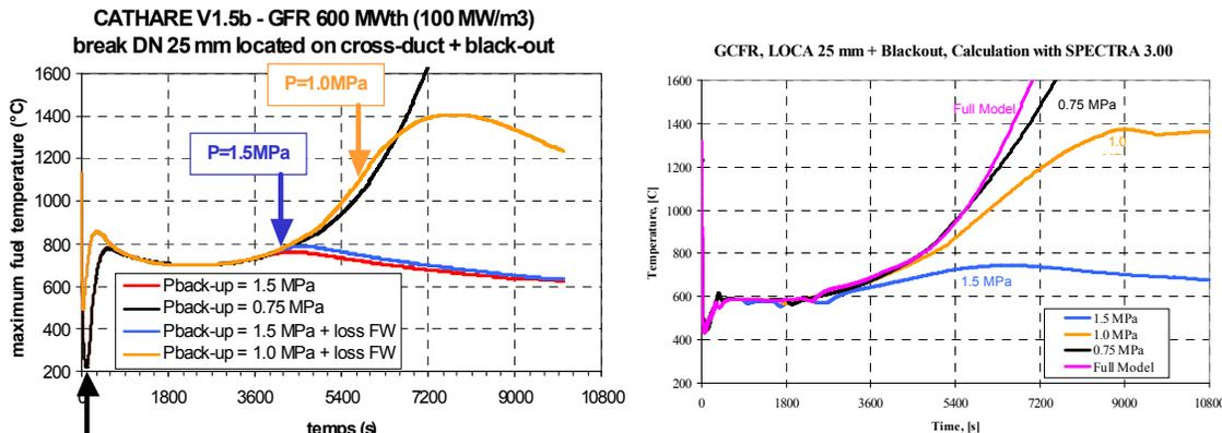
**Fig 3 Left: Maximum fuel temperature, LOCA D=25 mm - CATHARE results [8];
