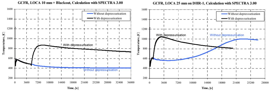
**Fig 6 Left: Maximum fuel temperature, LOCA 10 mm, SOPS.**
