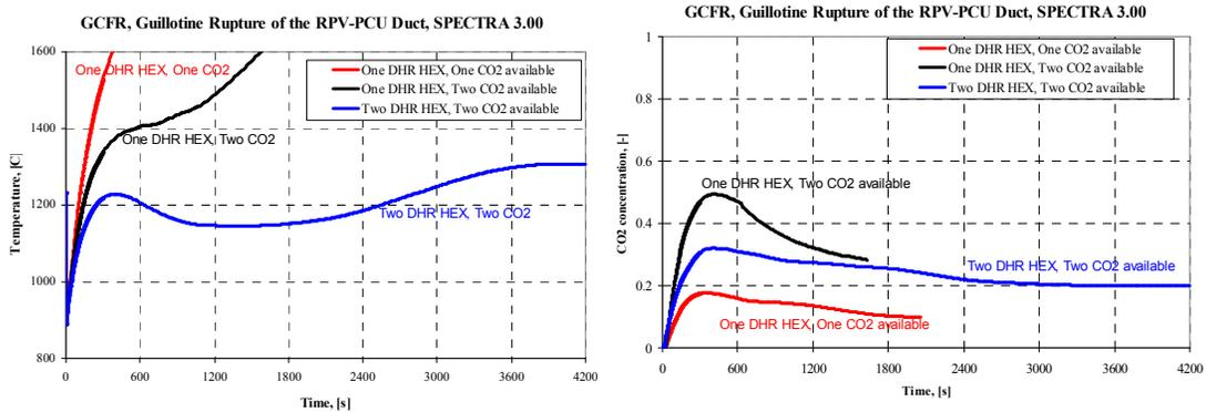
**Fig 8 Left: Maximum fuel temperature, rupture of the RPV-PCU duct.**
