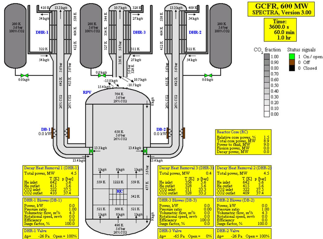
Fig 11 CO<sub>2</sub> concentrations at t = 3600 s. DHR-3 duct rupture, Case 3.
