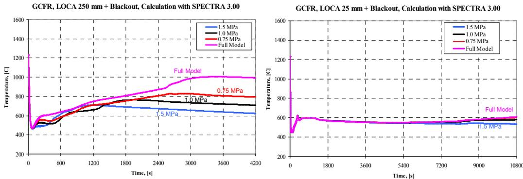
**Fig 5 Left: Maximum fuel temperature, LOCA 250 mm, SOPS.
