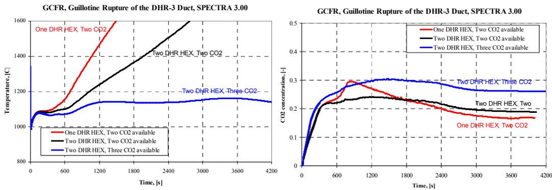
**Fig 10 Left: Maximum fuel temperature, rupture of the DHR-3 duct.
