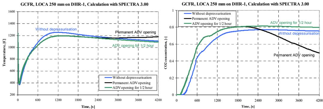
**Fig 7 Left: Maximum fuel temperature, 250 mm, near CO<sub>2</sub> injection.**
