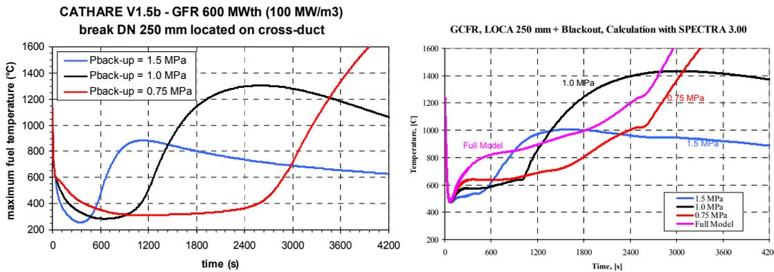
**Fig 2 Left: Maximum fuel temperature, LOCA D=250 mm - CATHARE results [8];
